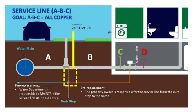
The shows responsibilities of the YWD and the homeowner for the water service line. Depending on the year built of you home and the age and material of the existing watermain, the service line may be lead, galvanized, plastic or copper. In 2023 The YWD has begun to replace the PWS (Public Water System) lead service lines.
